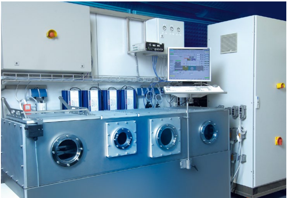
Fig. 4: VUV excimer plant of the Fraunhofer IFAM for activating and coating surfaces.
