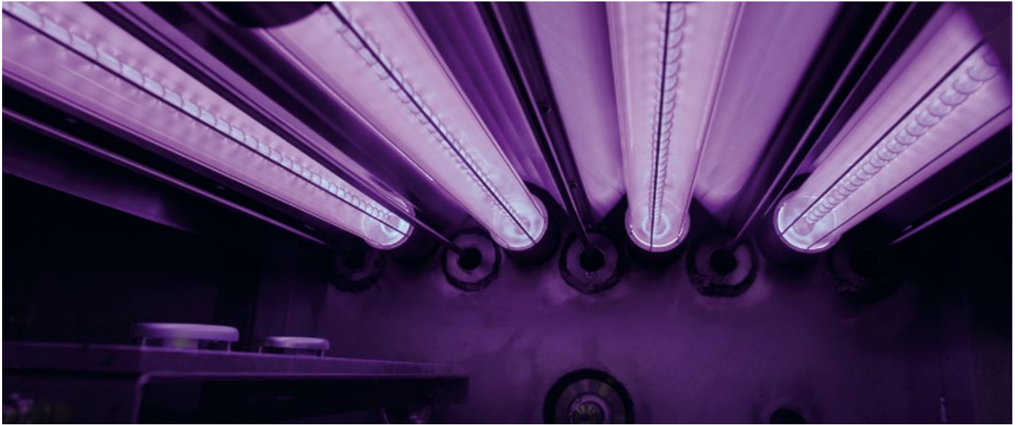
Fig. 5: Internal view of the VUV excimer plant.
