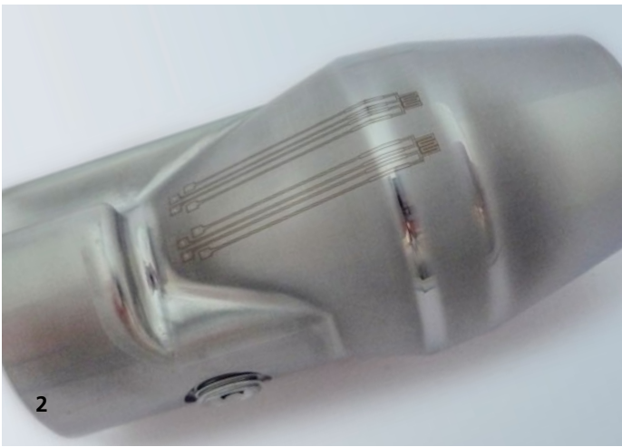
2 Mold core with two sensor structures on the surface.
